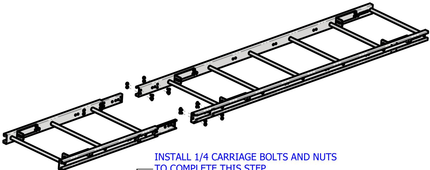
INSTALL 1/4 CARRIAGE BOLTS AND NUTS
